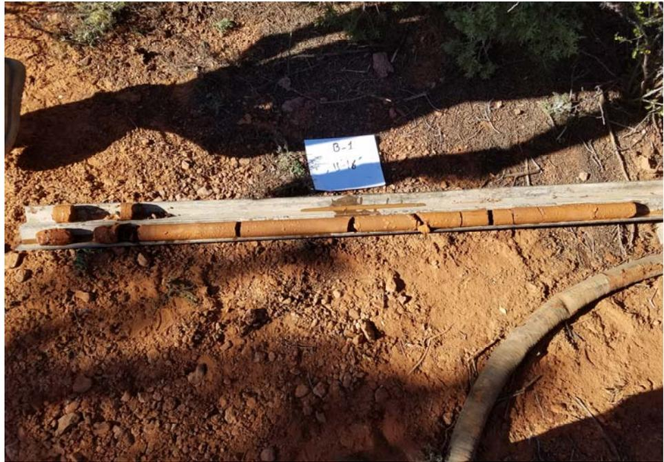
**Photograph 1:** Sample cores B-1, 11 through 16 feet.
