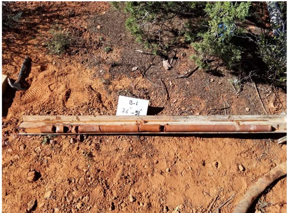
**Photograph 4:** Sample cores B-1, 26 through 31 feet.
