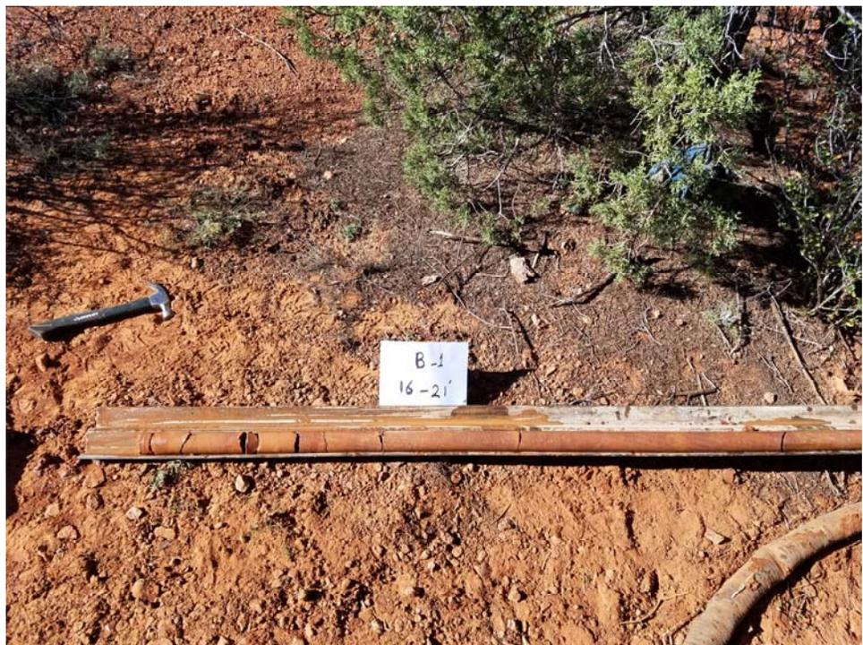
**Photograph 2:** Sample cores B-1, 16 through 21 feet.
