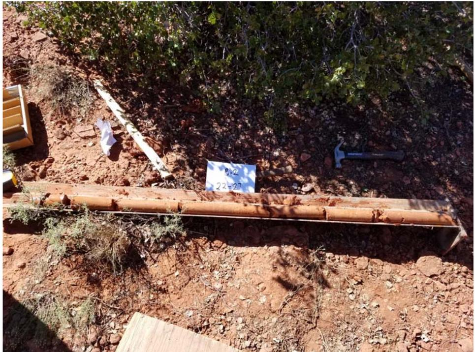
**Photograph 6:** Sample cores B-2, 22 through 27 feet.
