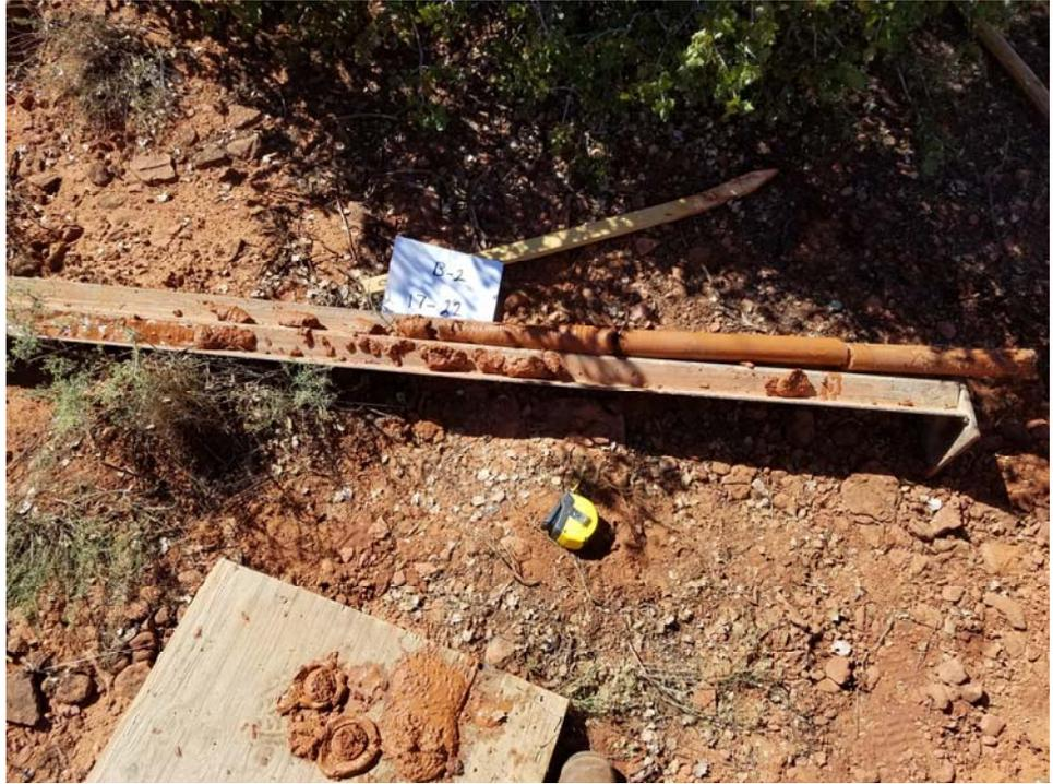
**Photograph 5:** Sample cores B-2, 17 through 22 feet.
